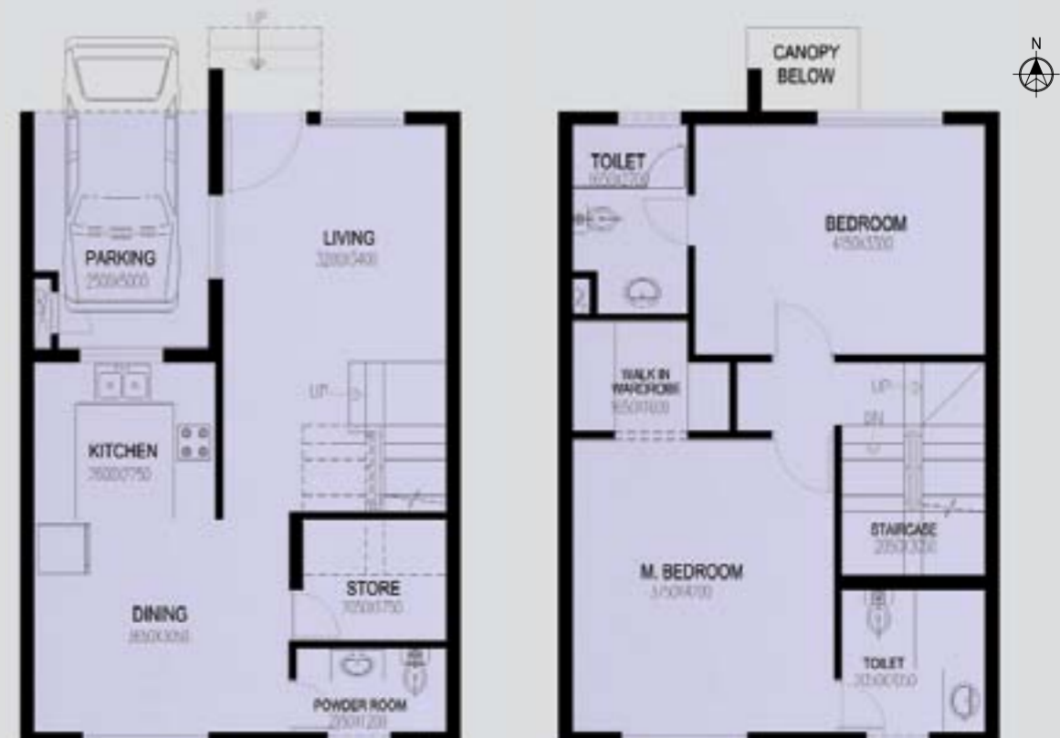
VILLAS 4-14 2BHK Plot Area =74.42 Sqm/801.06 Sft Build-up Area /Saleable Area =116.18 Sqm/1250.56 Sft GROUND FLOOR PLAN
