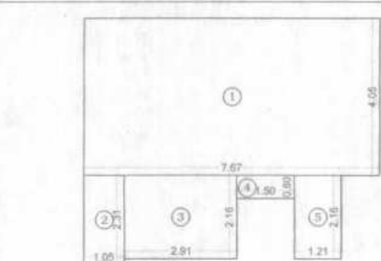
RERA CARPET AREA DIAGRAM OF FLAT NO.7 (1ST TO 12TH FLOOR) SCALE = 1:100
