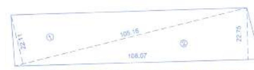
ROAD WIDENING AREA TRIANGULATION SCALE-1:1000
