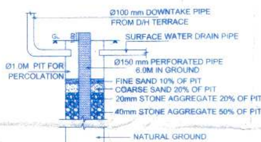
RAIN WATER HARVESTING DETAILS
