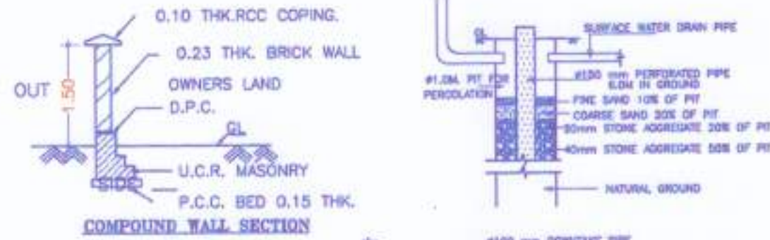
RAIN WATER HARVESTING DETAILS
