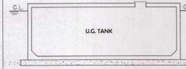
SECTION THROUGH UNDER GROUND TANK SCALE: 1:50
