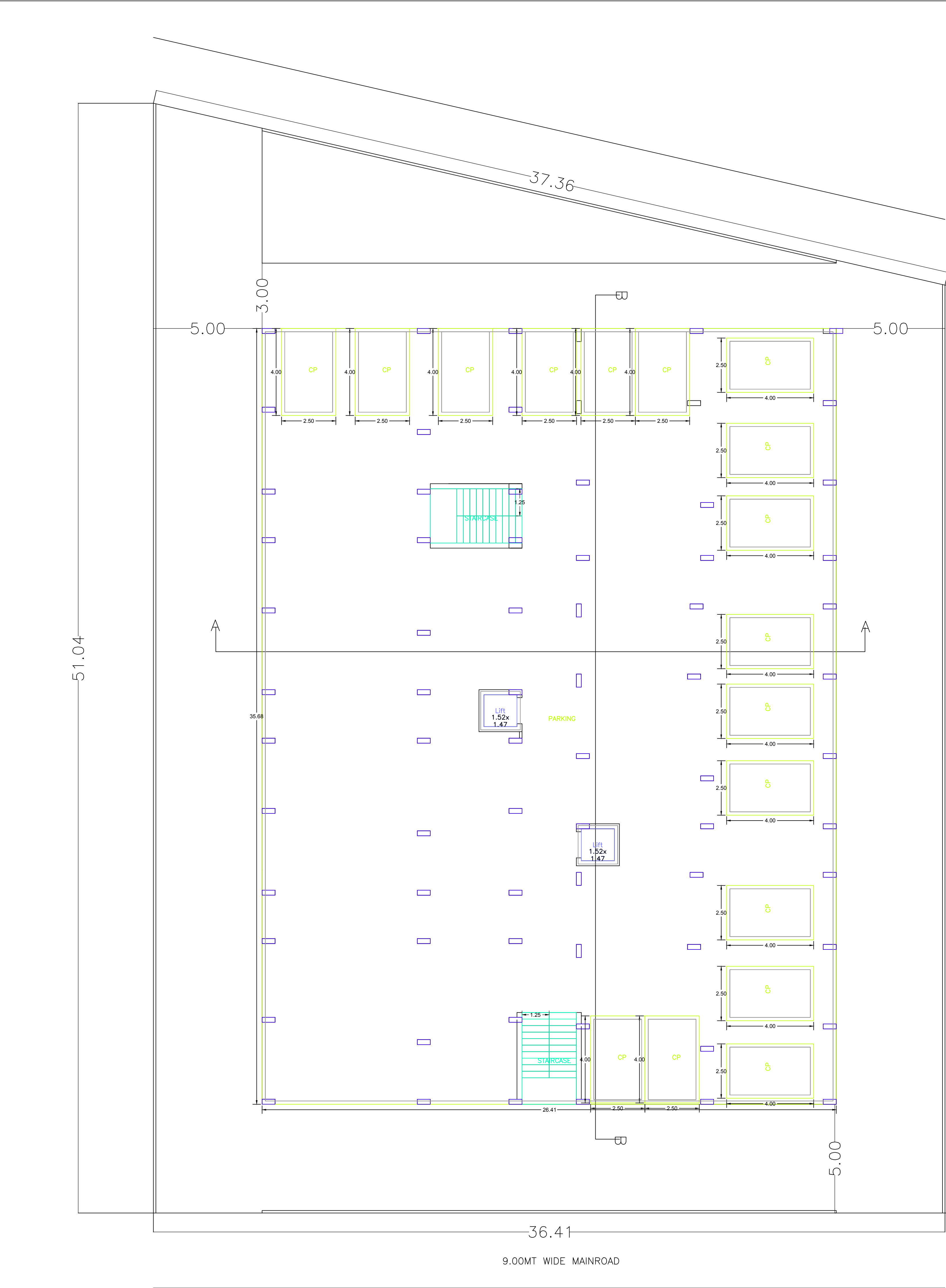
STILT FLOOR PLAN (SCALE 1:100)
