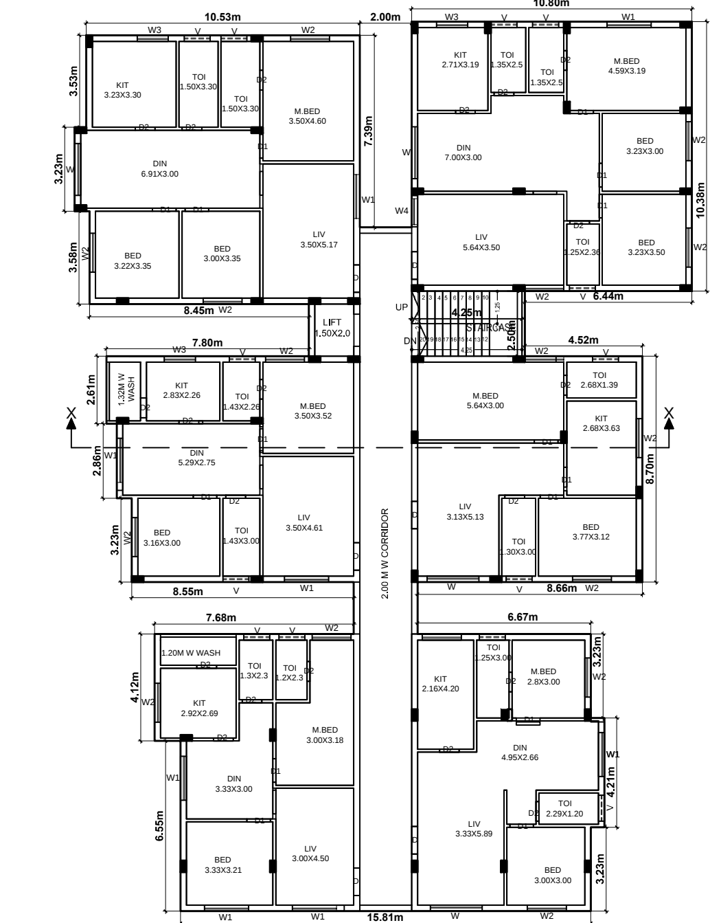
PRO. TYPICAL FLOOR PLAN (FIRST, THIRD, FOURTH & FIFTH FLOORS) (SCALE 1:200)
