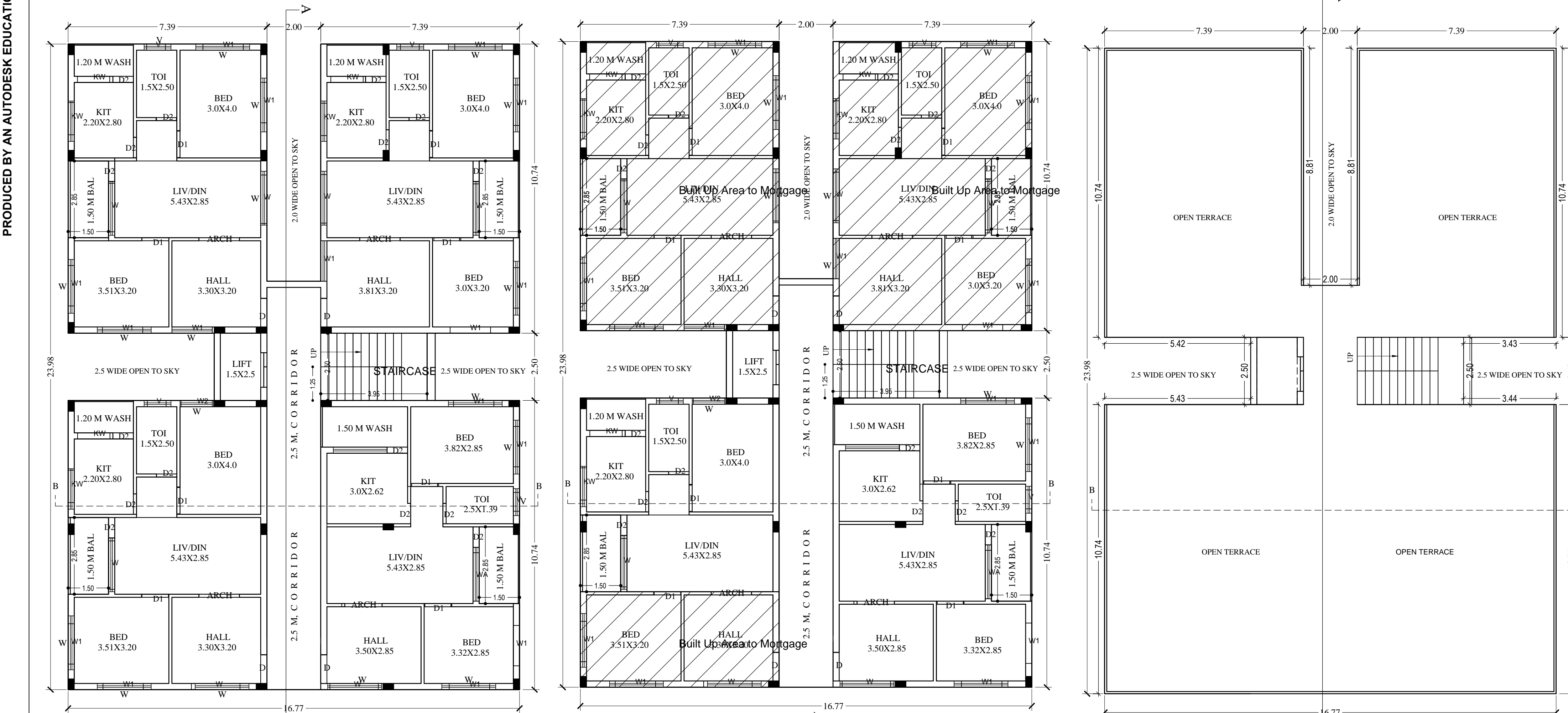
TYPICAL FLOOR PLAN 2nd, 3rd, 4th & 5th FLOORS (SCALE 1:100)
