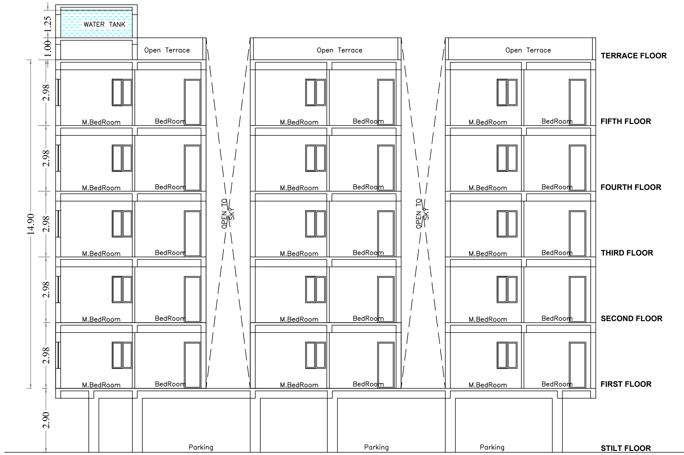
SECTION 'Y-Y' SCALE (1:100)
