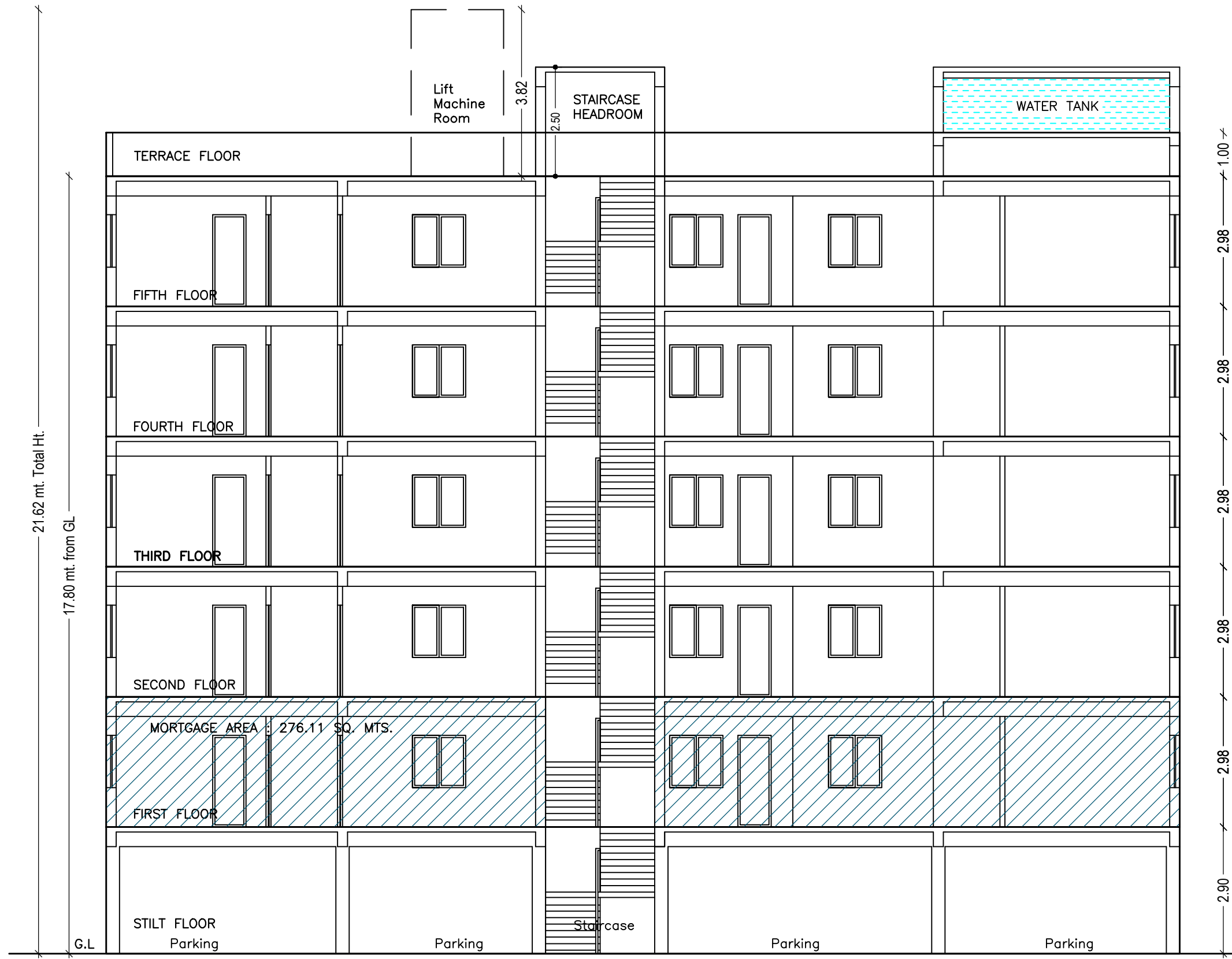
SECTION 'X-X' SCALE (1:100)
