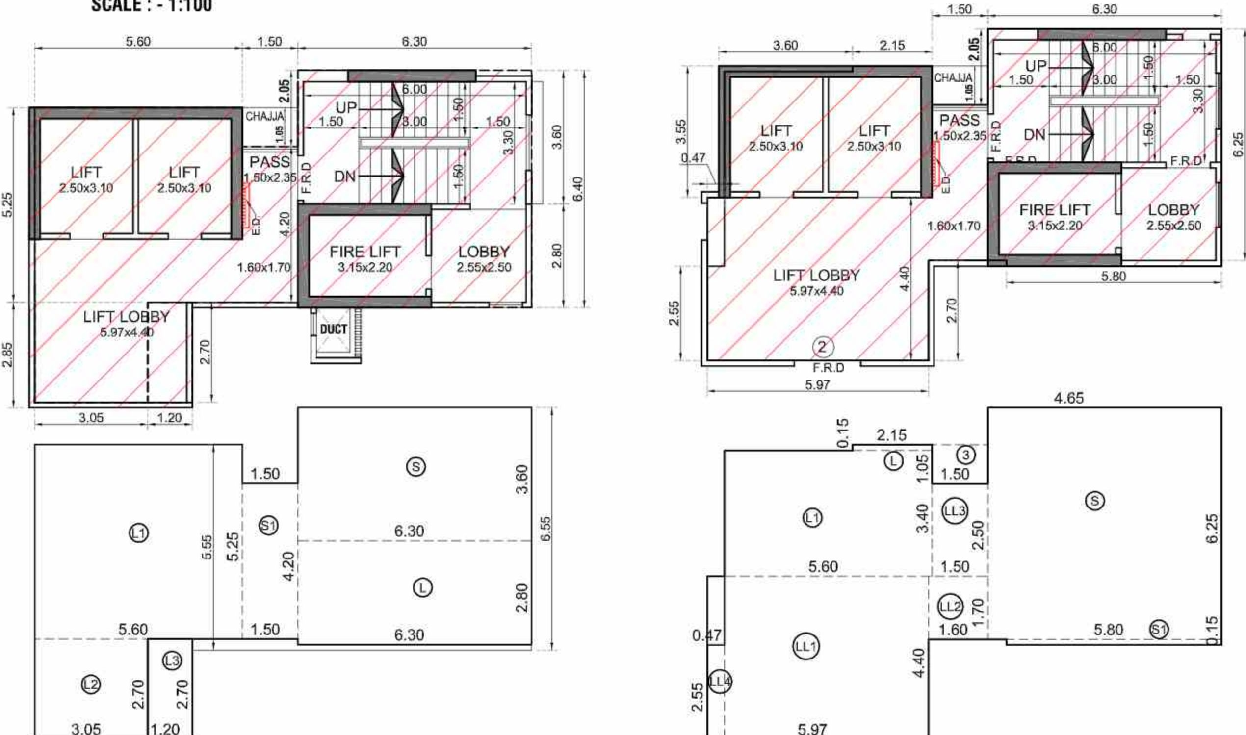
STAIRCASE PREMIUM AREA DIAGRAM FOR 4TH TO 10TH FLOOR SCALE = 1:100
