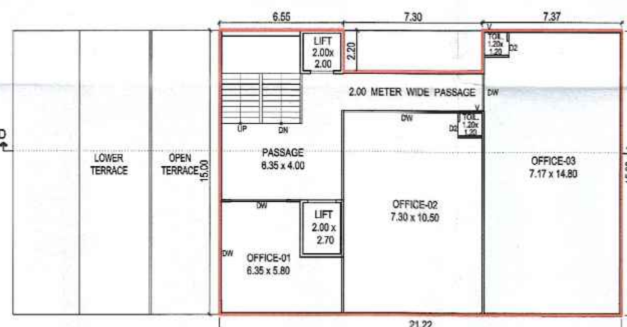
7TH FLOOR PLAN (TOWER : 02) B. A. : 302.17 SQ.MT. / DEDU. : STAIR + LIFT = 66.28 SQ.MT. / F.S.I. AREA : 235.89 SQ.MT.
