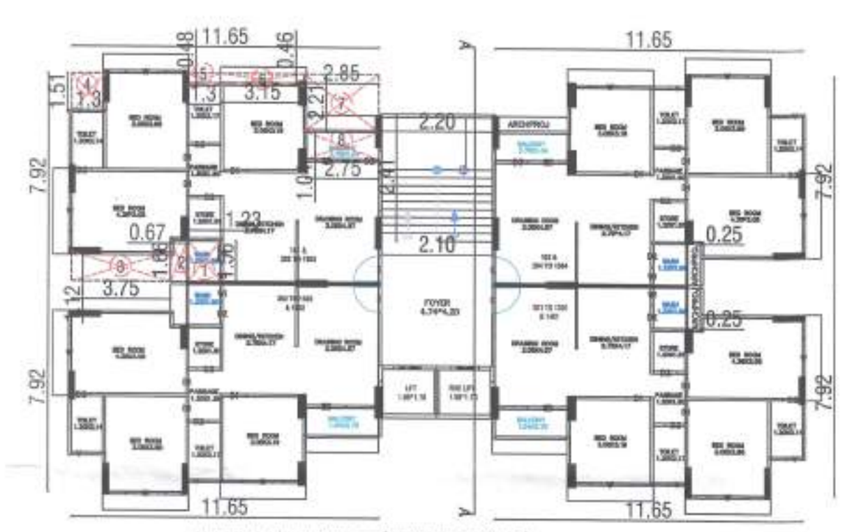
TYPICAL FLOOR AREA CALC. SHEET (FOR TWO UNITS OF 1401, 1402)
